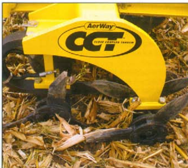
VERTICAL AND LATERAL TILLAGE. Low-concavity blade design on the True-Tandem 330 Turbo (left), offset AerWay ShatterTines (right) and other designs allow vertical tillage implements to move soil vertically and laterally for a uniform seedbed and maximum soil fracture.
