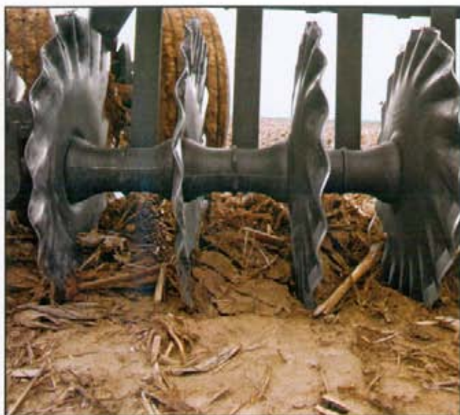
VERTICAL AND LATERAL TILLAGE. Low-concavity blade design on the True-Tandem 330 Turbo (left), offset AerWay ShatterTines (right) and other designs allow vertical tillage implements to move soil vertically and laterally for a uniform seedbed and maximum soil fracture.
